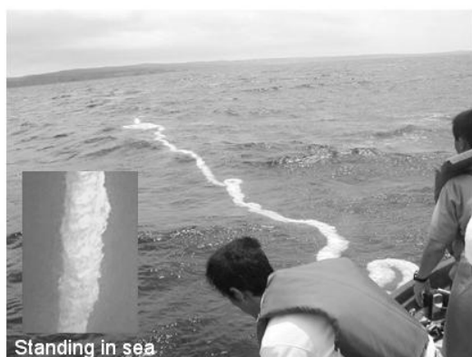
Figure 6 Recovery of braid adsorbent in marine experiment at Okinawa.
